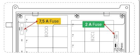
Step 7: Insert Fuse. Insert the supplied main 7.5 A fuse in its position at the top left corner. The device connected to the AUX port will power on now.
